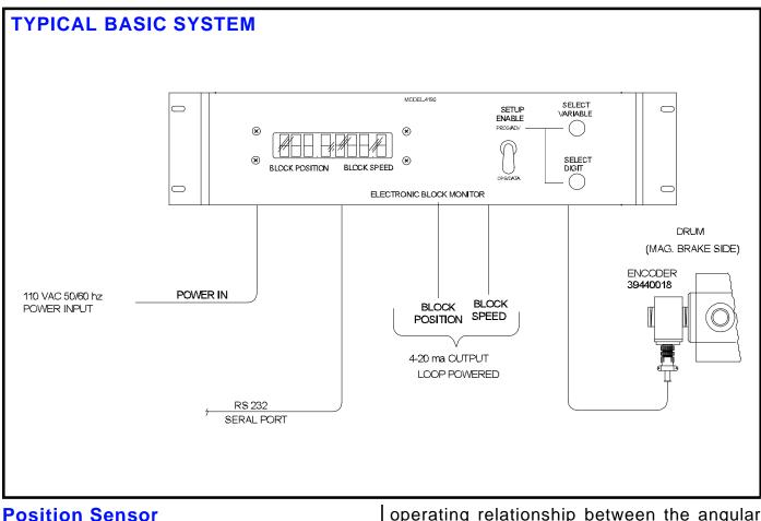
The relationship between the linear movement of the wire line and the angular position of the drawworks drum is predictable, repeatable and can be calculated using the diameter and the length of the drum and the size of the wire line. By
